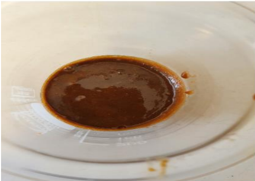
Oily deposits from inside the bend section
