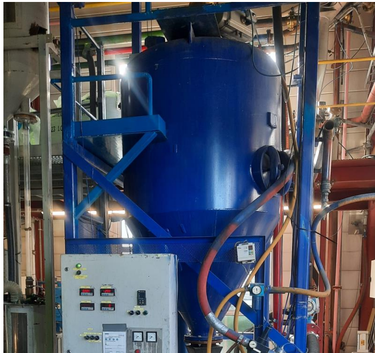
Figure 3.3: Picture of the pellet feeding tank.
