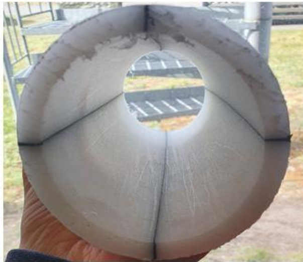
Figure 5.23: Internal view of the cleaned bend cross-section after erosion test.
