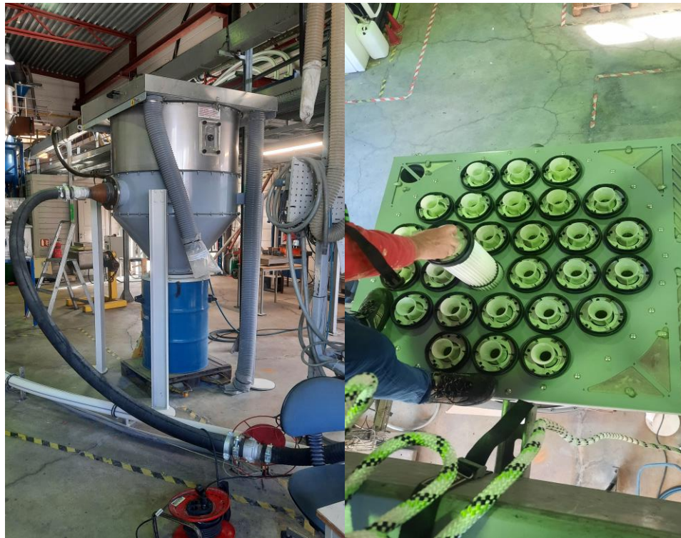
Figure 3.7: Gas-solid separator - A 28 filter cartridge system.
