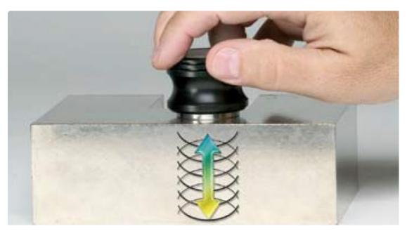
Figure 20 Ultrasonic testing in metal sheet to measure the thickness of metal.
