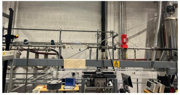
Figure 16 Experimental setup for multiphase flow.
