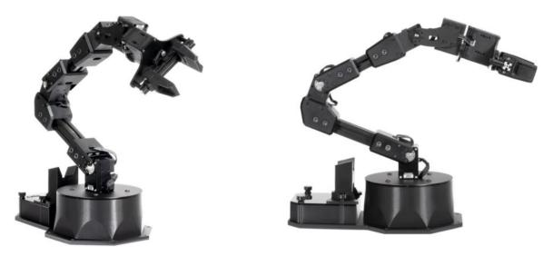
Figure 1: ReactorX 150 robotic arm manipulator
