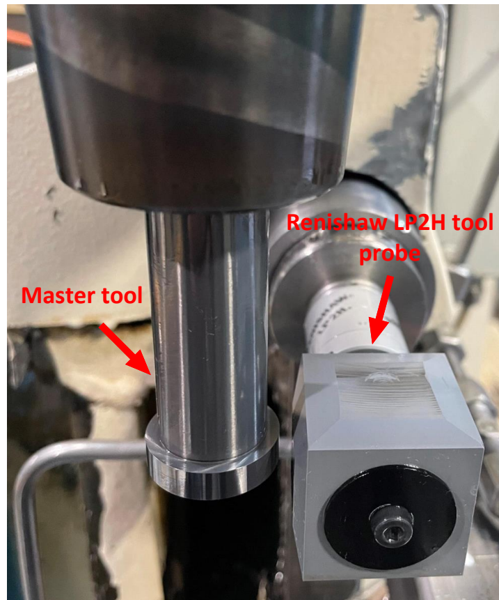
Figure 2.4: Master tool for calibration and the Renishaw LP2H tool probe with a 30x30mm cube. Photo: Walter Johansson
