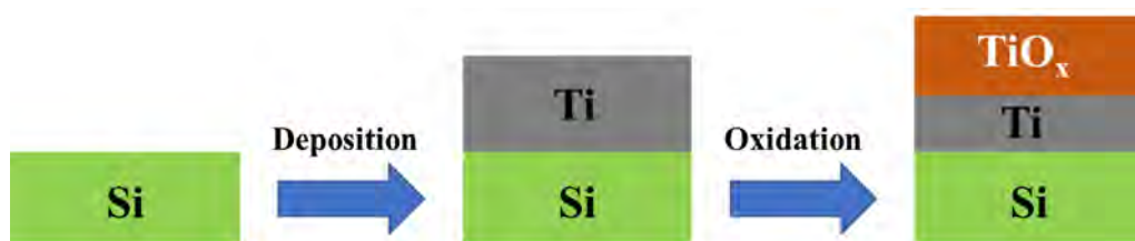
Fig. S13. Schematic illustration of the fabrication processes for the Ti-TiO x film composites on a plane substrate of silicon. The metallic Ti film was deposited by E-beam. The thickness of the flat Ti film is 300 nm, with the roughness of Ra: 84 nm; Rq: 255 nm, on the substrate of silicon. The as-deposited Ti was followed by the various thermal oxidation temperatures (400, 450, 500, 550, 600, 650 °C) for 5 h in a tube furnace with the controlled flowing of oxygen gas. The roughness was measured by the interferometer (Wyko NT9100).
