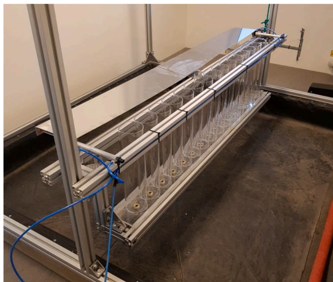
Fig. 2. Measurement of the actual water flow/flux by using a patternator.
