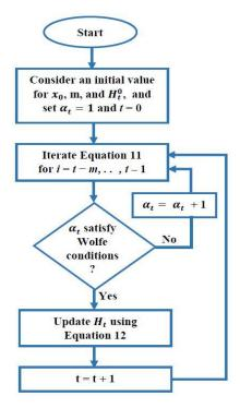
Figure 2. Flow chart of the limited-memory Broyden-Fletcher-Goldfarb-Shanno (LM-BFGS) algorithm.
