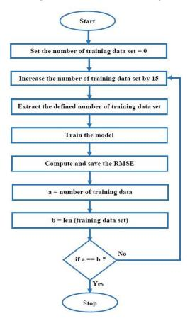
Figure 3. Flow chart of the optimization process.
