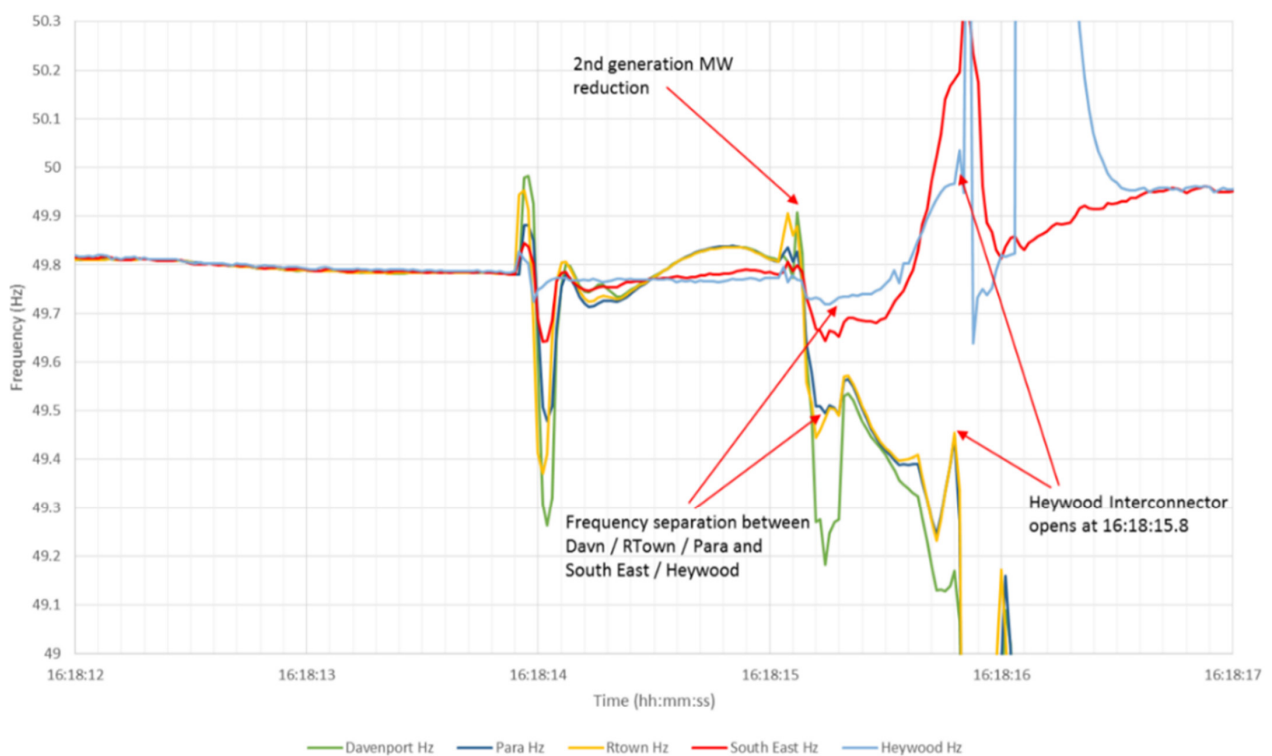
Figure 9. Dynamics of frequency in various nodes of South Australian grid during the failure on 28 September 2016 [73].
