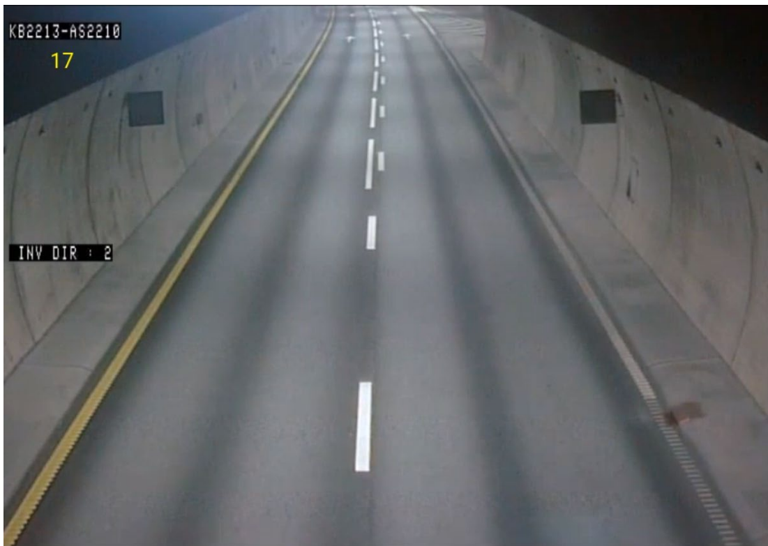
Figure 3-6 Inverse direction is triggered by AID-system
