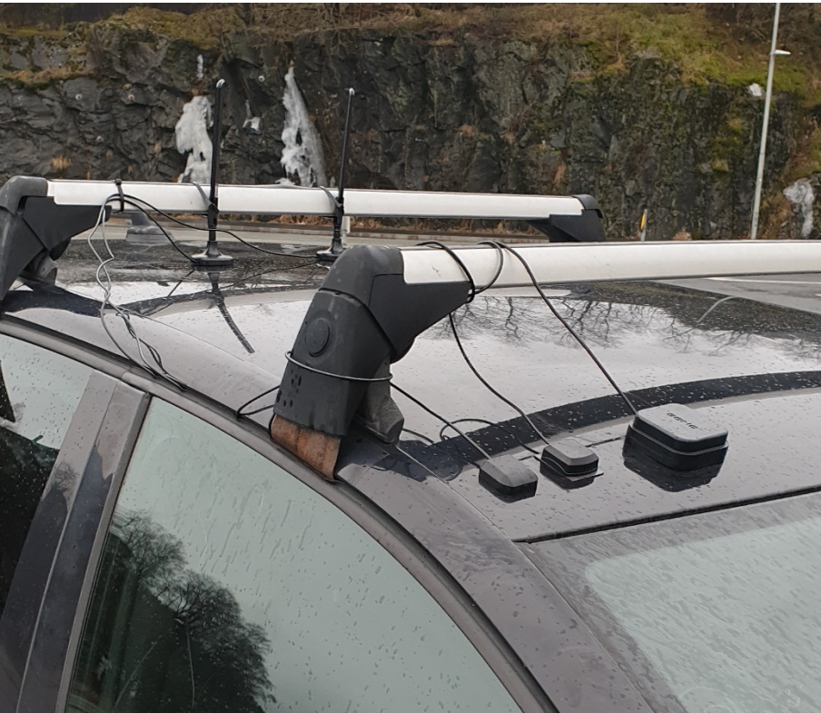
Figure 4-9 Placement of GNSS-antennas and cellular network antennas on the car roof
