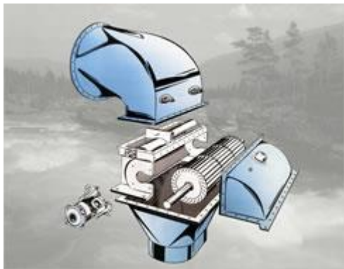
Figur 6: Cross flow turbin [9]
