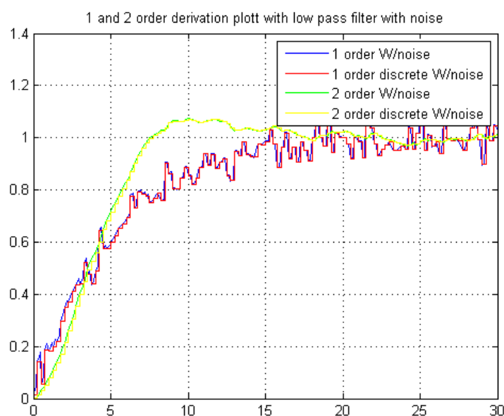
Figure 2 - Ramp response of derivate TF with noise
