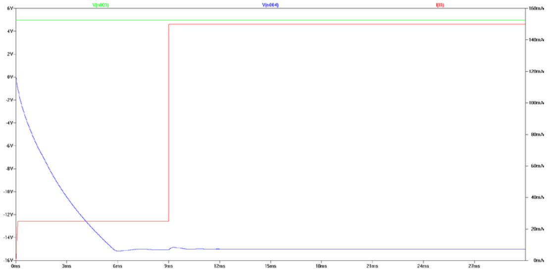
Figure 165 - Load test for -15 V power supply
