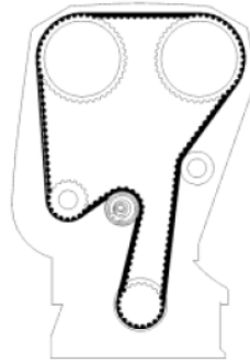
Figure 124 - Timing belt 95
