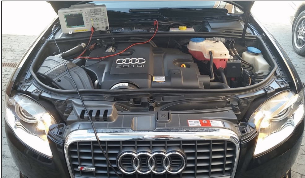
Figure 133 - Audi A4 battery voltage testing
