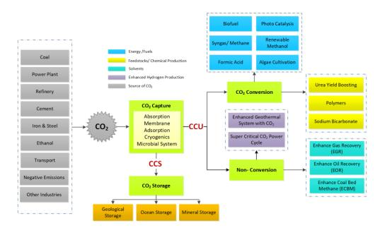
Figure 3. The CCUS schematic diagram.
