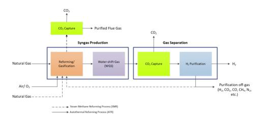
Figure 1. The blue hydrogen process flow: SMR and ATR.
