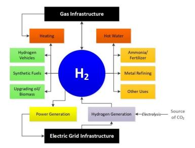
Figure 5. The hydrogen utilization options.
