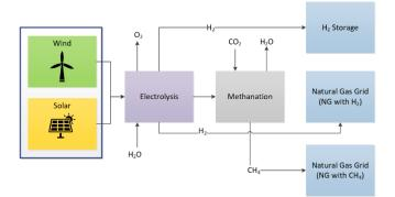
Figure 2. The green hydrogen schematic.
