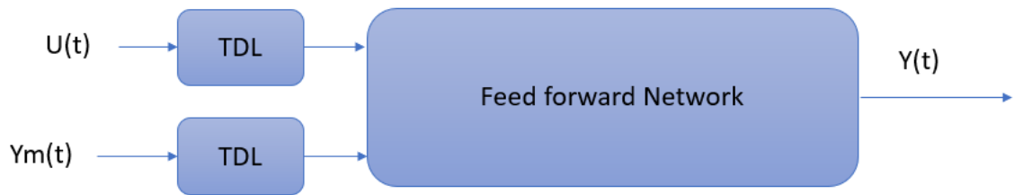
Figure 9-3 Parallel series architecture NARX neural network with tapped time delay line. Y(t) is predicted output. Y_m(t) is measured output from process.
