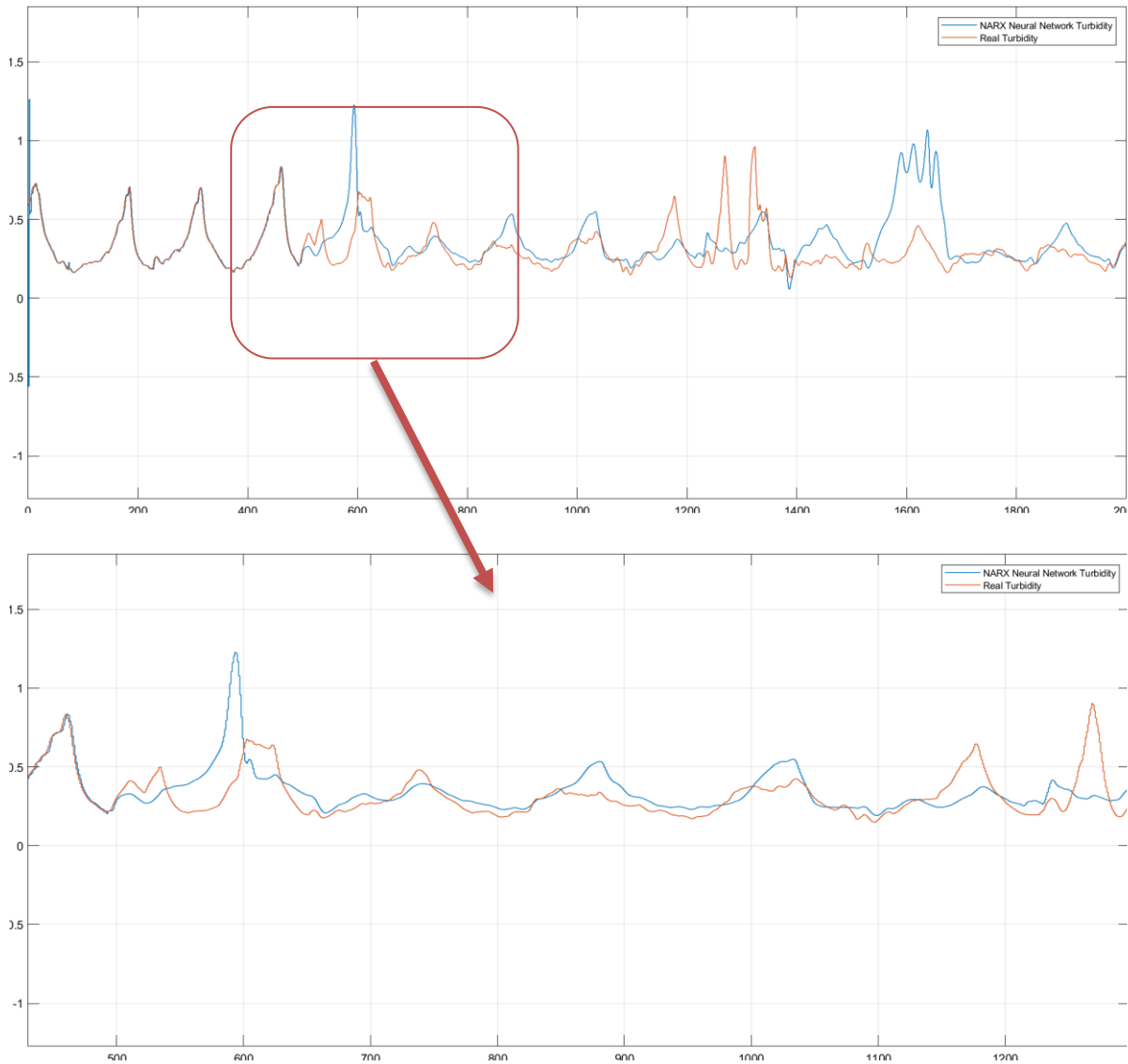
Figure 10-13 NARX ANN model response for MISO. Parallel series NARX architecture from 0 to 500, parallel NARX ANN architecture from 500 to the end, the inputs are PIX, PAX, POL, Inflow, PH, Temp. x-axis is the number of samples, the time between samples is 10 minutes. Y-axis is a turbidity FTU. All values are normalized.
