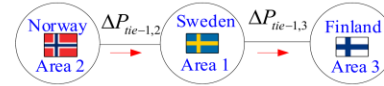
Fig. 4. Simplified model of the NPS. \Delta P_{tie} is used to represent the incremental active power change during a system frequency event
