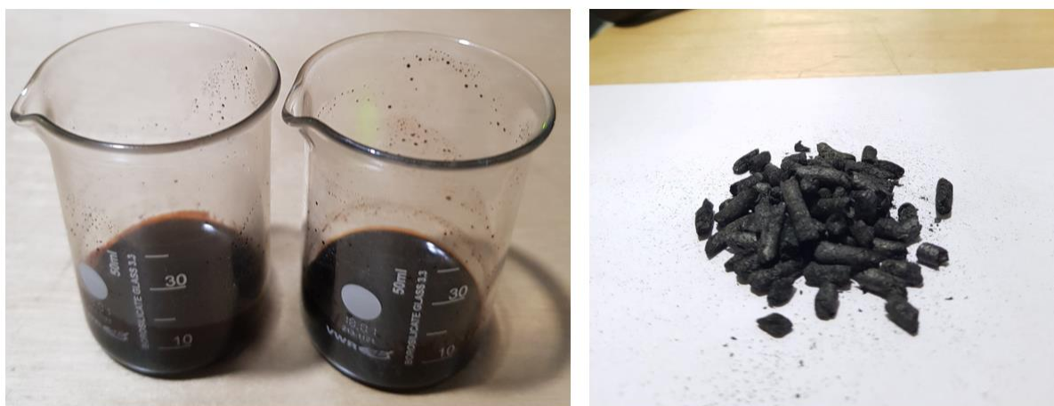
Figure 6.1 Tar and char produced from pyrolysis of wood pellets at 500°C.
