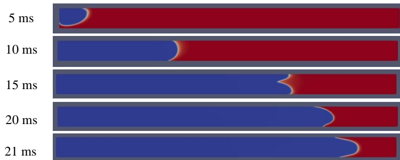
Figure 4.9. Flame propagation sequences in homogeneous H 2 -air mixture-equivalence ratio 1.2
