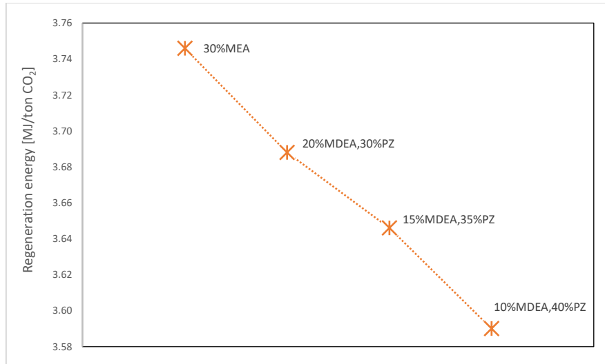
Figure 6.3: Investigation of MDEA+PZ blend in term of regeneration energy for standard process comparing with MEA
