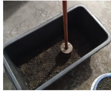
B. Crushing Leca manually using a weight attached to a metal rod.
