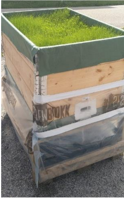
Figure 5: Prototype of the intensive green roof test model fully developed. Made of EURO pallets and pallet collars as main construction material. Planted vegetation (Spire Hestebeite), drainage hole (white square in the bottom middle) and a water collector tub underneath (black tub).
