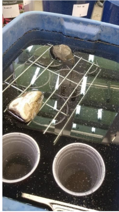
B. A metal grid with rocks was placed on top of the product samples to avoid them from floating and rolling over.
