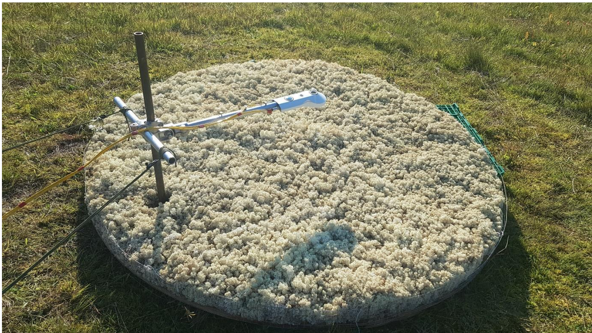
Figure 2.4 The subject board consisting of C. stellaris with a radiometer
