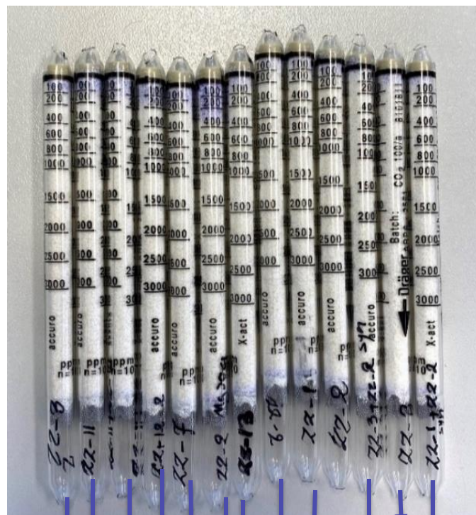
Figure3- 6: CO 2 evolution test on pure cultures, probable stimulators, and synergistic samples
