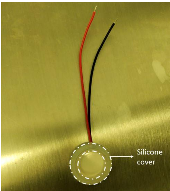
Figure 13: Piezoelectric transducer with silicone cover
