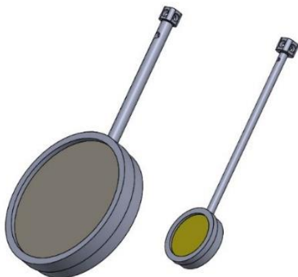
Figure 27b: Holders with transducer and sample attached in it
