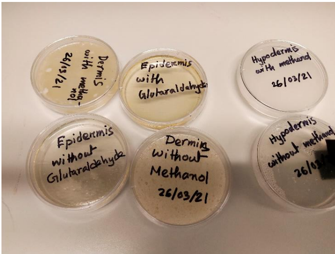
Figure 9: Different phantom gel layers in petry dishes
