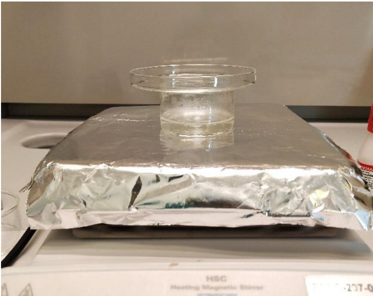
Figure 10: Phantom skin sample on the hotplate (turned on) covered with a lid to avoid evaporation of the chemical solution
