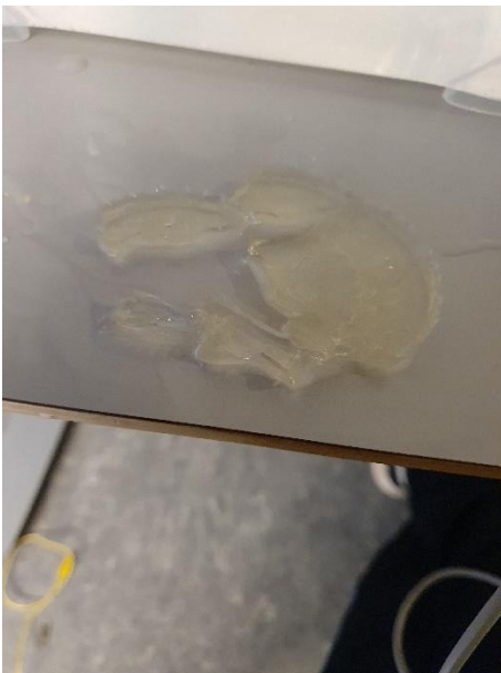
Figure 26: Damaged phantom sample
