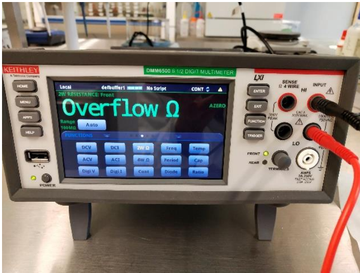
Figure 7: Multimeter used for resistance measurement
