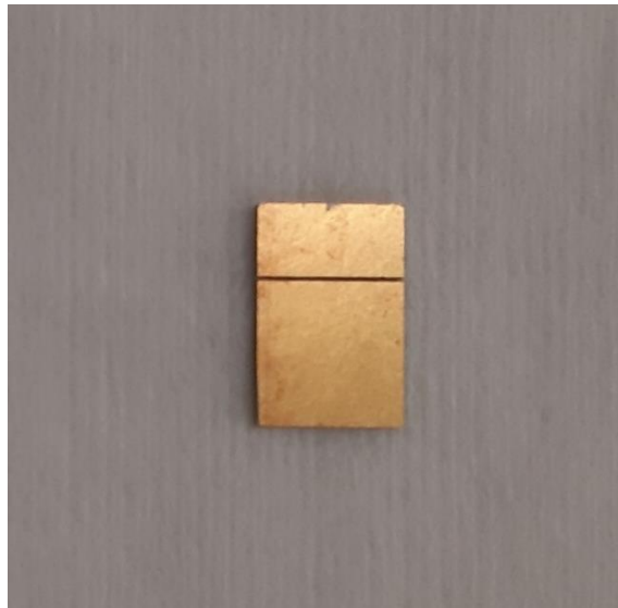
Figure 3.11: Pz27 sample from above after creating wrap around.
