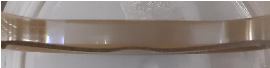
Figure 4.19: The cross section of the test sample with 40 µm spheres without Byk, SoS2. Practically all of the spheres are gathered in the bottom of the sample due to sedimentation.
