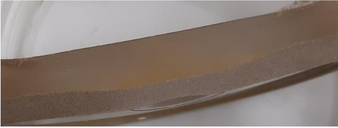
Figure 4.20: The cross section of the test sample 20 \mu\text{m} spheres with Byk, SoS3.
