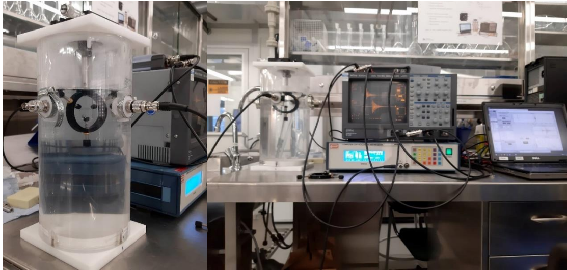
Figure 3.4: Speed of sound setup; measurement setup (left) and oscilloscope, signal source and computer setup (right).
