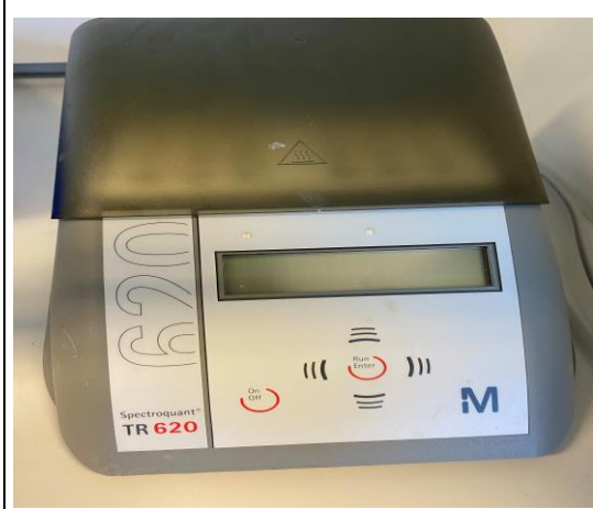
Thermoreactor TR620 used for heating the COD cells to 148°C.
