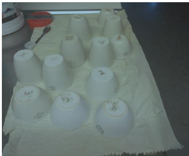
Porcelain basins used for keeping sample for the measurement of TS, VS, TSS, VSS.
