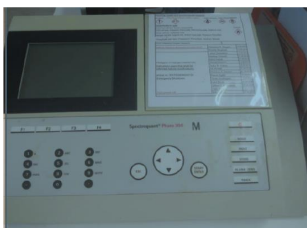
A spectroquant pharo 300 used for measuring the concentrations of COD, NH 4 -N, NO 2 -N, NO 3 -N, and alkalinity.
