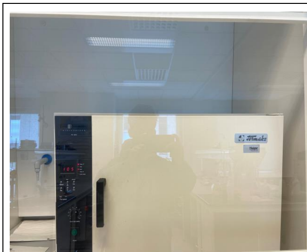
Oven at temperature 105°C for drying TS, and TSS.
