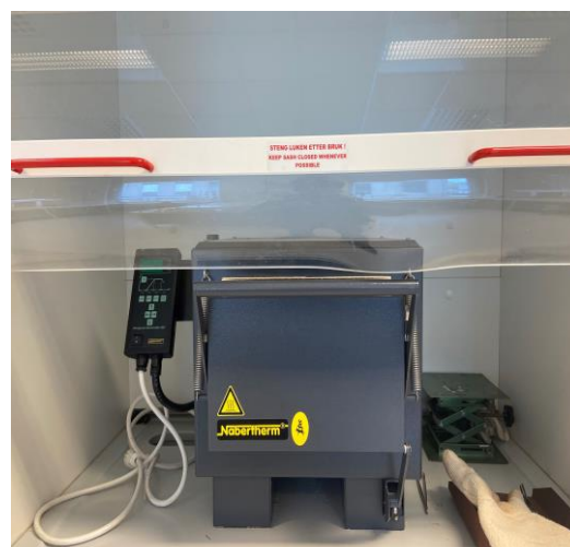
Muffle furnace at temperature 550°C to ignite volatile solids.
