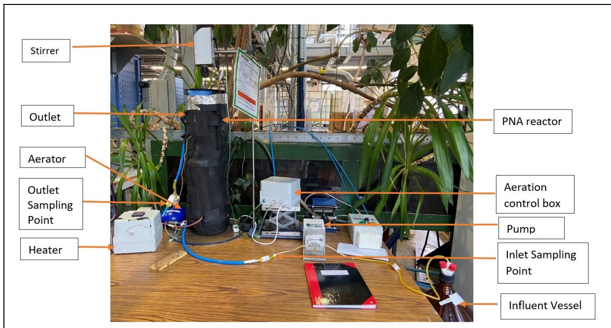
Figure 3.1: Experimental reactor set-up at USN.
