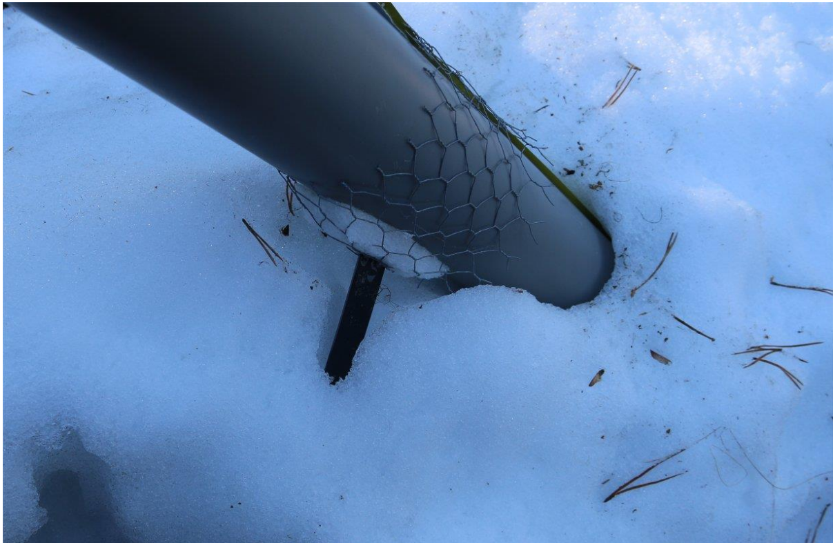
Figure 4.1: Snow contracts and recedes from the moisture sensor when the temperature gets too high
