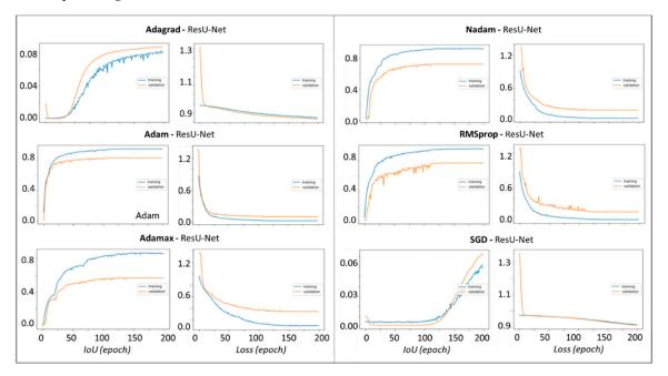
**Figure 6.** Fluctuation of IOU and loss function values after 200 epochs of ResU-Net models using six optimizer functions.
