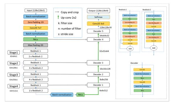
Figure 4. ResU-Net structure for training a model to classify coastal wetland ecosystem types.
