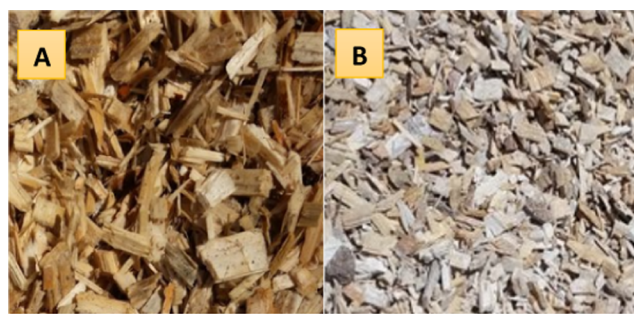
Figure 1. Two different samples of wood chips: without (A) and with (B) additive from spruce forest residues.
