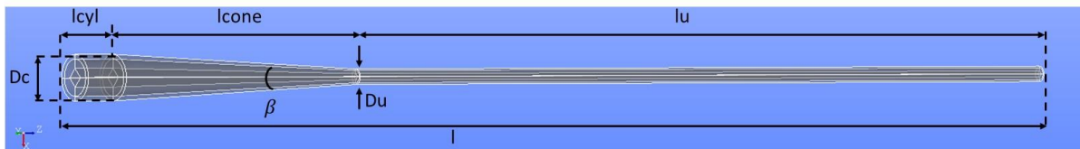
Figure 4.2: Hydrocyclone geometry adapted from Young et al. (1994, p. 40)
