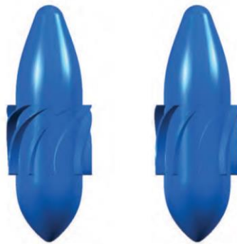
Figure 2.9: Strong swirl element (left) and weak swirl element (right). (Campen, 2014, p. 72)
