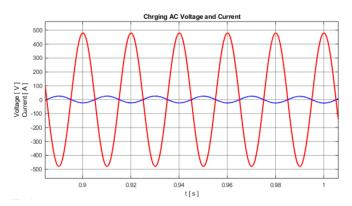
Figure 6.10: AC voltage and current when power flows from the grid to the EV battery.
