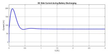
Figure 5.25: DC discharging current at phase angle 10°.
