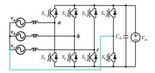
Figure 3.4: Three-phase four-leg bidirectional AC-DC converter [33].
