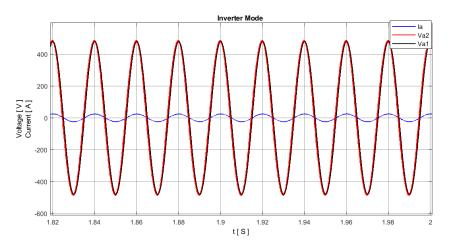
Figure 5.22: AC voltage generated by the inverter, AC grid voltage, and current (25 A).
