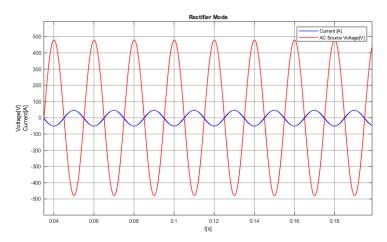
Figure 5.4: AC voltage and current under rectifier mode with a 1° phase angle.
