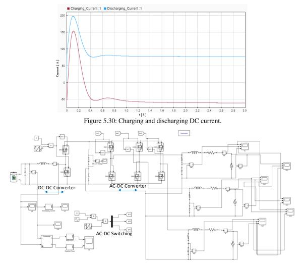
Figure 5.31: Simulation model proposed for EV charger without galvanic isolation.
