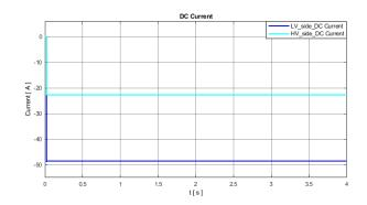
Figure 6.4: Average charging DC current in the LV and HV side $\varphi = 2.16^{\circ}$ .
