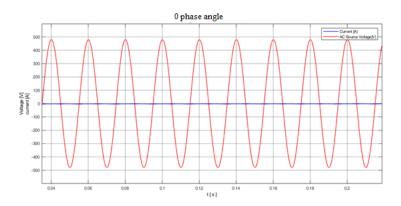
Figure 5.3: When the phase shift is 0° in a sine wave, no current flow.
