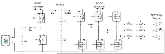
Figure 5.1: A simplified two-stage bidirectional EV charger without galvanic isolation.
