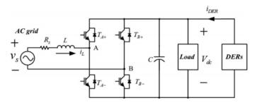
Figure 3.1: A bidirectional single-phase ac-dc converter in a load connected to dc microgrid and the grid [34]
