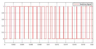
Figure 5.12: Generated gate pulse switching.
