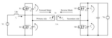
Figure 3.12: Half-bridge bidirectional DC-DC converter [50].
