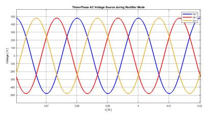
Figure 5.14: Three-phase grid voltages during charging.
