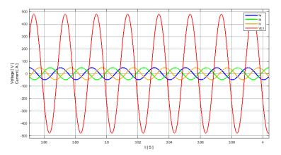
Figure 5.19: The three-phase current and voltage in phase B during charging.
