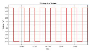
Figure 6.2: Low voltage side AC square voltage.
