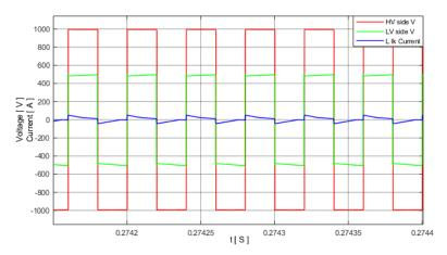
Figure 6.14: HV and LV side voltages and inductor current displaying soft switching.
