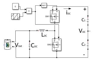
Figure 5.8: Bidirectional DC-DC converter.
