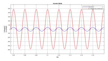
Figure 5.5: AC voltage and current under inverter mode with a 1° phase angle.
