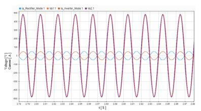
Figure 5.29: AC voltage and current for rectifier nad inverter mode in phase A.
