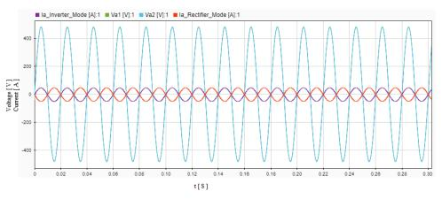
Figure 5.7: AC voltage and current for both rectifier and inverter mode.
