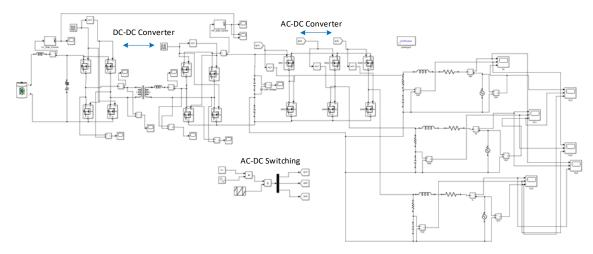
Figure 6.15: Simulation model proposed for EV charger with galvanic isolation.
