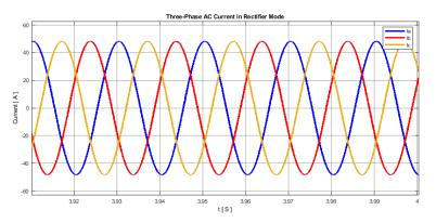
Figure 5.15: Three-phase grid currents during charging.
