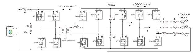
Figure 6.7: A two-stage bidirectional EV charger with galvanic isolation.
