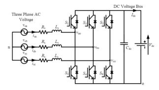
Figure 3.3: Three-phase two-level H-bridge bidirectional three-phase AC-DC converter [38].
