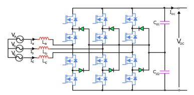
Figure 3.5: Three-phase three-level neutral point clamp AC-DC converter [30].
