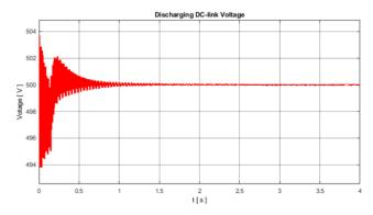
Figure 6.11: DC-link voltage during discharging.
