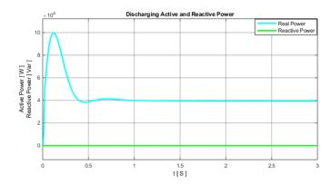
Figure 5.28: Active and reactive power injecting from the battery to the grid.
