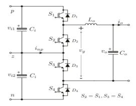
Figure 3.10: Bidirectional three-level DC-DC converter [43].
