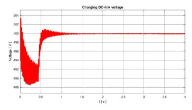
Figure 6.8: DC-link voltage during charging.
