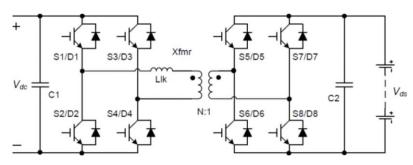
Figure 3.11: Bidirectional full-bridge DC-DC converter based on two voltage-fed [45].
