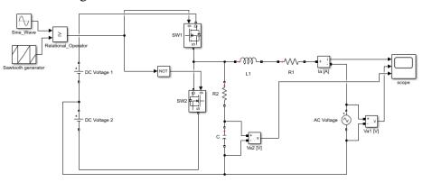
Figure 5.2: Half-bridge single-phase bidirectional AC-DC converter.
