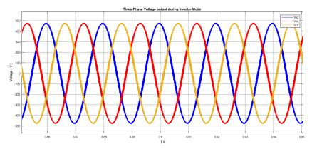
Figure 5.23: Three-phase AC voltage produced by the bidirectional AC-DC converter during discharging.
