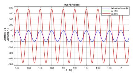
Figure 5.6: AC voltage and current under inverter mode with a 2° phase angle.
