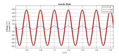
Figure 5.21: AC voltage generated by the inverter, AC grid voltage, and AC current (50 A).
