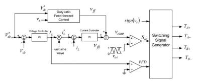
Figure 3.2: Control scheme for the simplified PWM switching [34].
