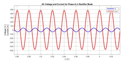
Figure 5.13: AC side voltage and current in phase A during charging.
