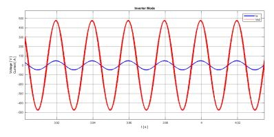
Figure 5.20: AC voltage and current converted by the bidirectional AC-DC converter during discharging.
