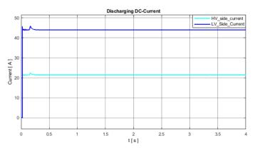
Figure 6.12: Average discharging DC current in the high and low voltage side of the DC-DC converter.
