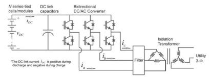
Figure 3.6: Single-stage three-phase bidirectional AC-DC converter [10].
