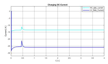
Figure 6.9: Average charging DC current in the high and low voltage side of the DC converter.
