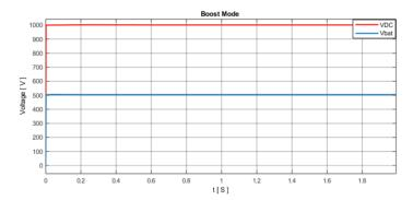
Figure 5.10: Input and Output voltages of the bidirectional DC-DC converter in Boost mode.
