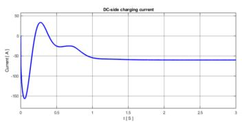
Figure 5.16: Battery DC charging current.
