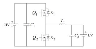
Figure 3.9: Buck-boost bidirectional DC-DC converter [42].
