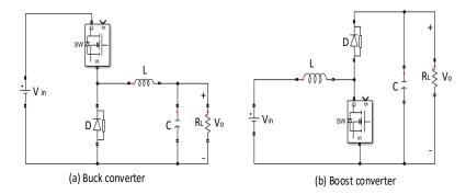
Figure 3.8: Unidirectional buck and boost converters.
