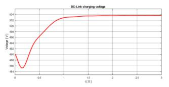
Figure 5.17: Center-taped DC link voltage during rectifier mode.
