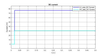
Figure 6.6: Average discharging DC current in the LV and HV side  $\varphi=5^{\circ}$ .
