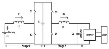
Figure 3.7: Cascade bidirectional DC-DC converter topology[40].
