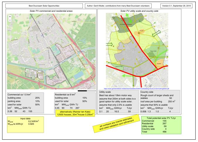
Fig. 6. The estimates for solar potential are using maps of residential, commrcial and countryside areas (original figure is A3 size)
