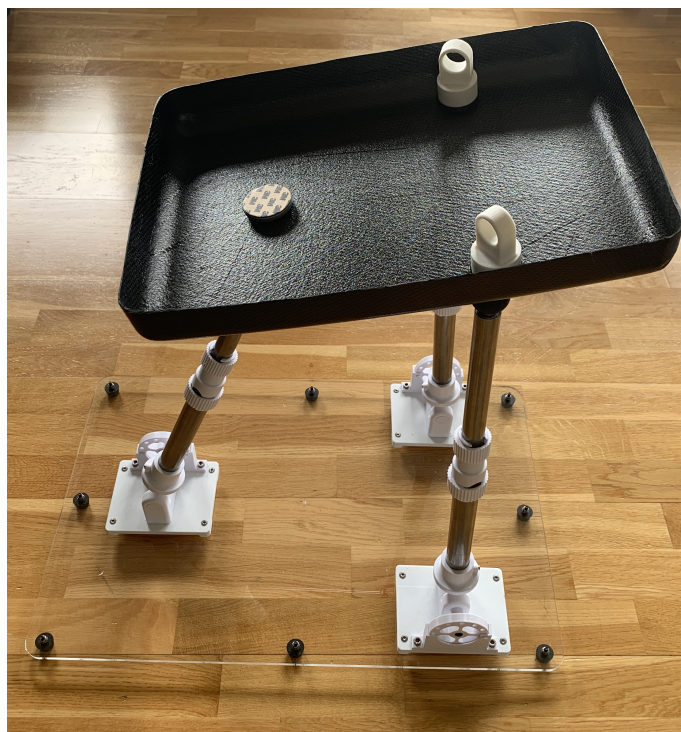
Figure 93: Fixture prototype V6.0 - Fixture Holding Composite Panel
