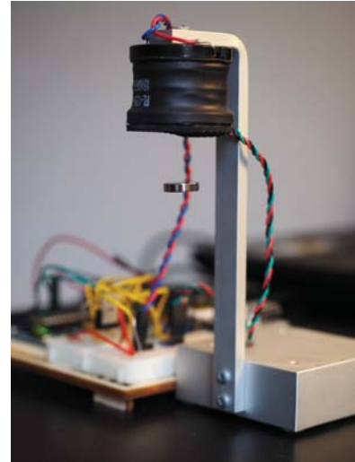
Figure 8. Arduino controlled electromagnetic levitation system.
