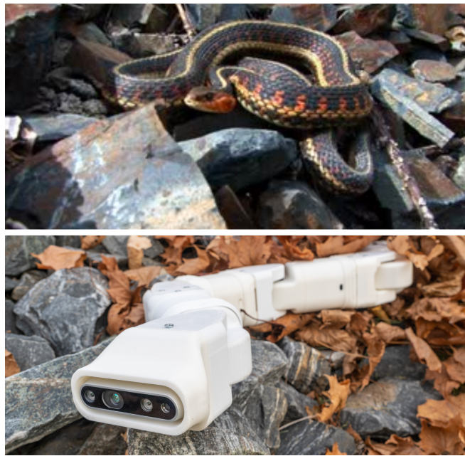
Fig. 1: A real snake locomoting in a cluttered environment (top); Serpens , the proposed low-cost ROS-based snake robot with series elastic actuator (SEA), precision torque control and a screw-less assembly mechanism (bottom).
