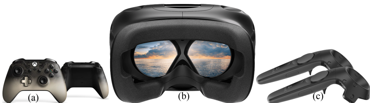
Figure 10: Simulator equipment. (a)Wireless XBOX controller for the 3D virtual reality simulator (Microsoft, 2019), and HTC VIVE VR system with (b) head mounted display and (c) hand controllers (VIVE, 2019) for the immersive virtual reality simulator.
