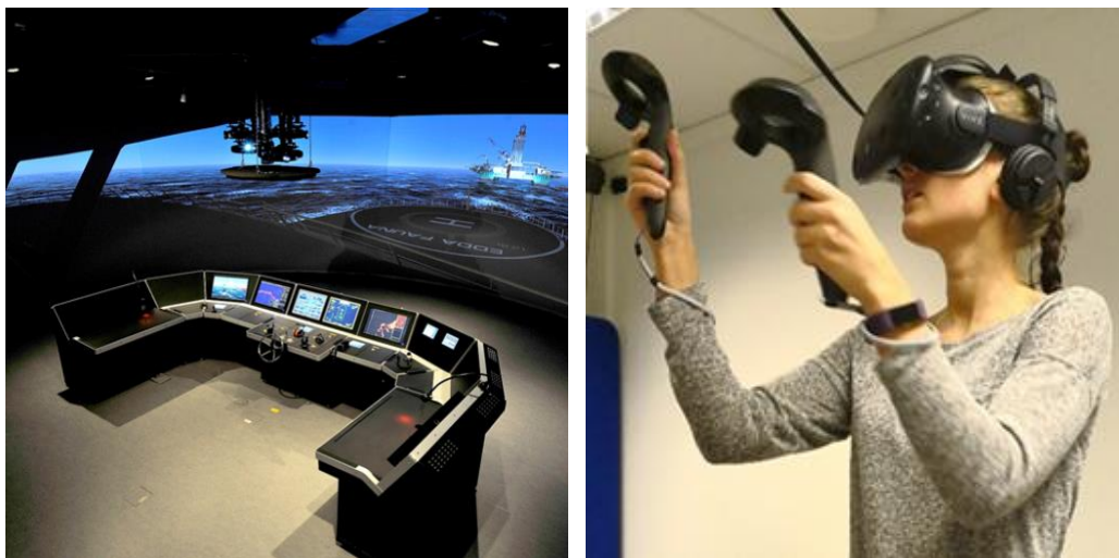
Figure 1. Full Mission Bridge Simulator System (left), virtual reality head-mounted displays (VR HMD) bridge simulator hardware (right).
