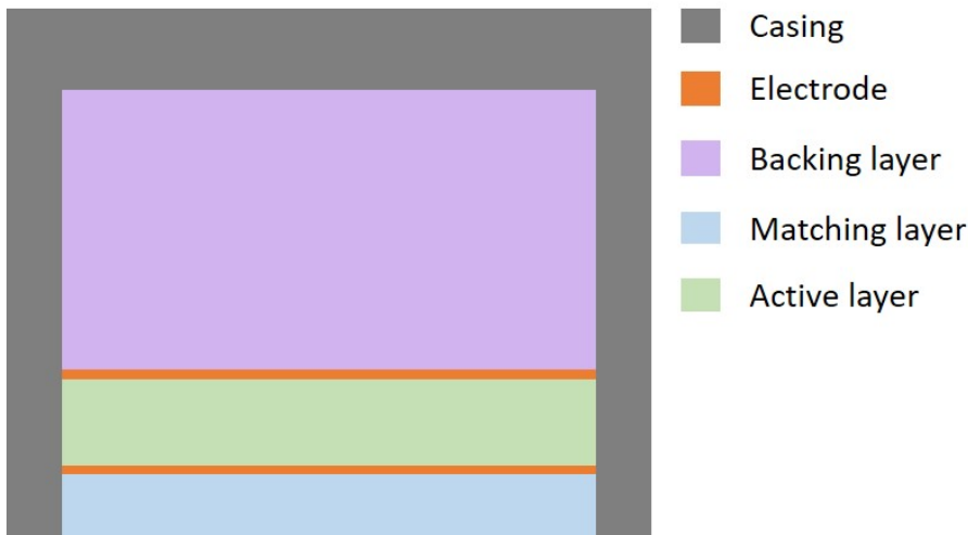
Figure 1.2: Simplified schematic of a transducer. The active layer can either be a piezoelectric material or a composite.
