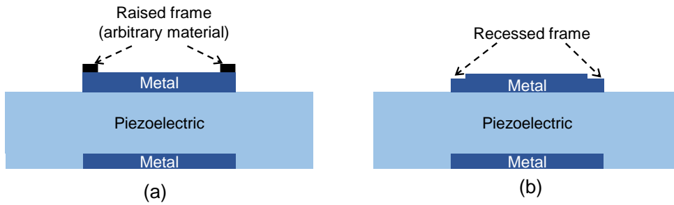
Figure 1.4: Frames in BAW resonators of type I (a) and type II (b) following the method proposed by Kaitila. The resonators are not drawn to scale.
