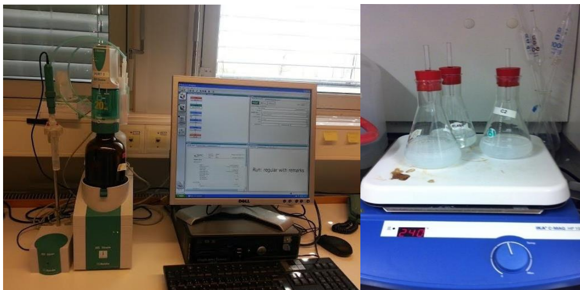
Figure 5.3: Sample analysis using titration method.
