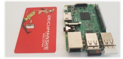
Figure 1.1 - The Raspberry Pi 3 Model B, with a size similar to a credit card.
