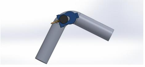
Figure 3.7: Ultrasonic sensor around the bending pipe (top view)
