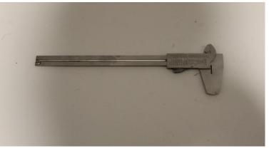
Figure 2: Vernier caliper
