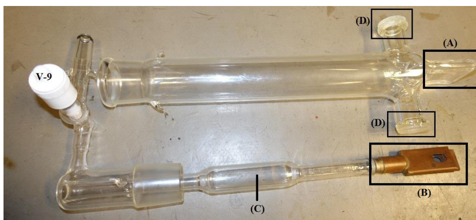
Figure 5.3: Photo of the self-designed cell for a low temperature experiment.
