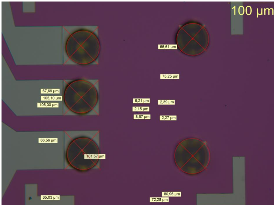
Figure 17: Stud bumps formed Si substrate, using 17.5 \mu\text{m} Au wire.
