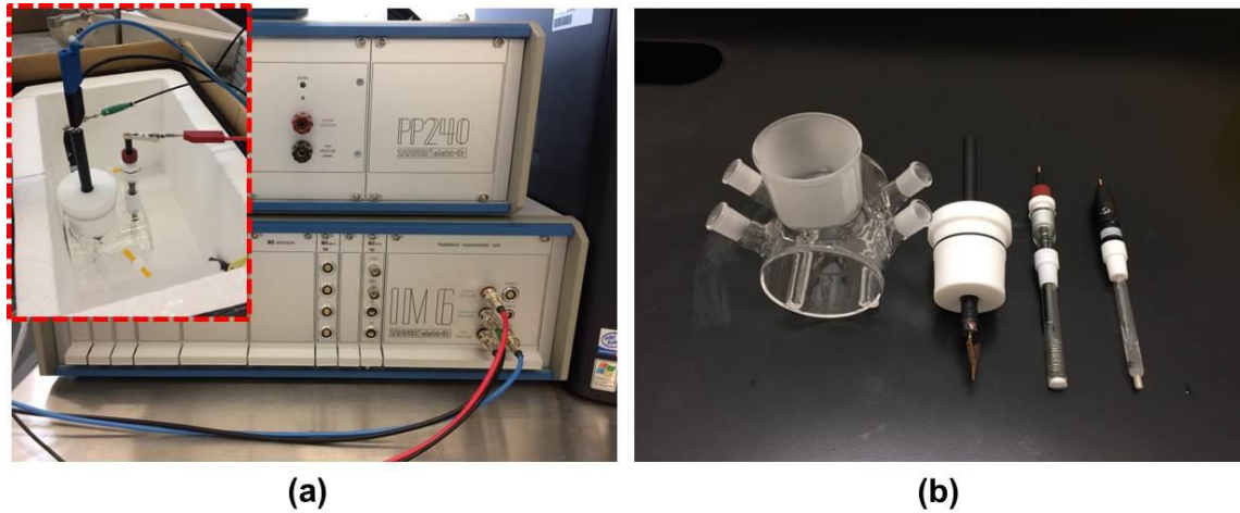
Figure 7 (a) Quartz reaction cell and (b) Zahner Elektrik impedance measurement unit. Inset: PEC measurement setup
