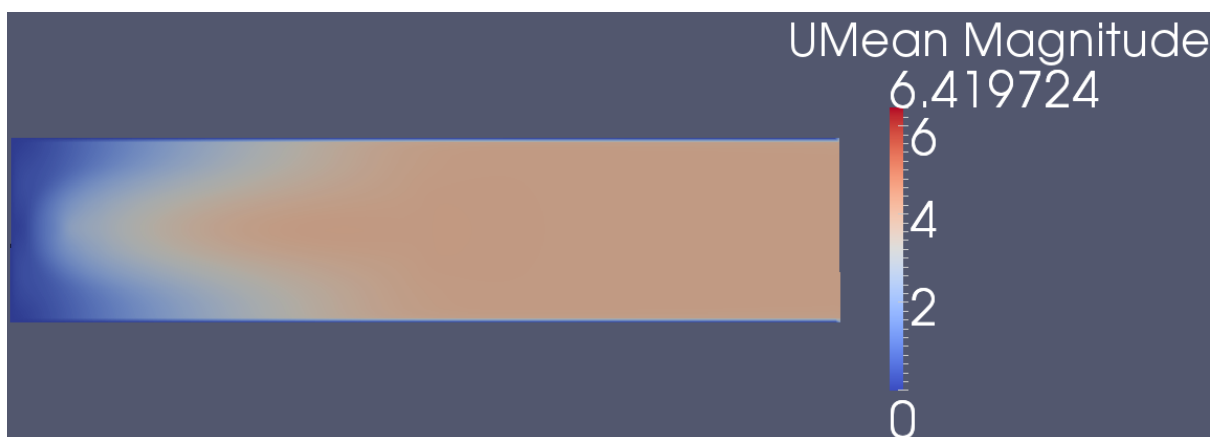
Figure 3-24: Average flame speed of premixed Li-ion LCO gas-air, at time step: 0.03.
