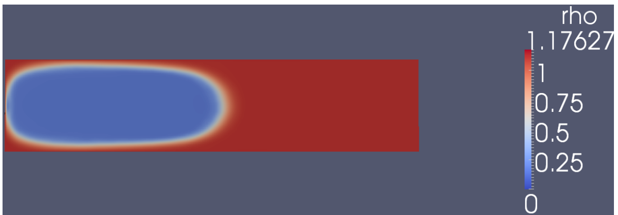
Figure 3-18: Density of premixed Li-ion LCO gas-air, at time step: 0.03.
