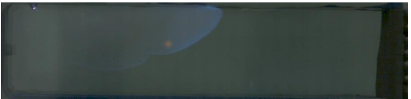
Figure 4-6: Premixed methane-air mixture, presumably lean. Printscreen of the flame front 0.0475 s from the position in Figure 4-5.
