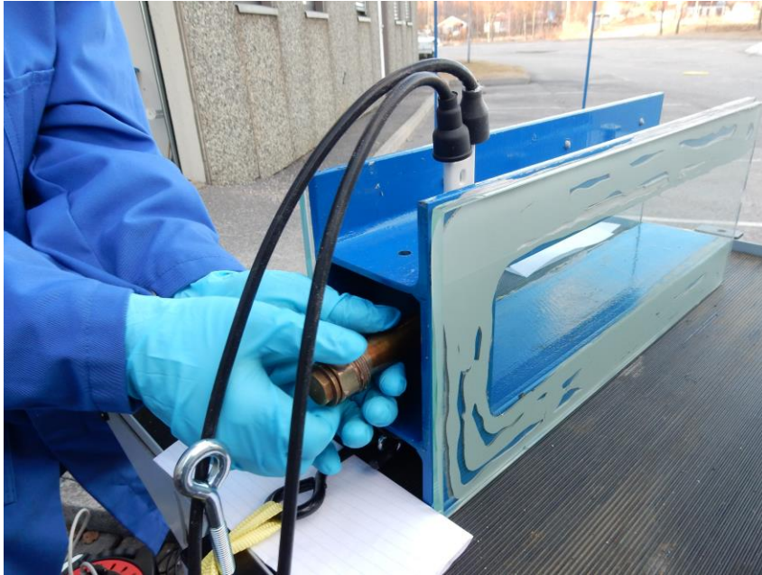
Figure 4-2: Picture of the battery-holster being mounted on the channel.
