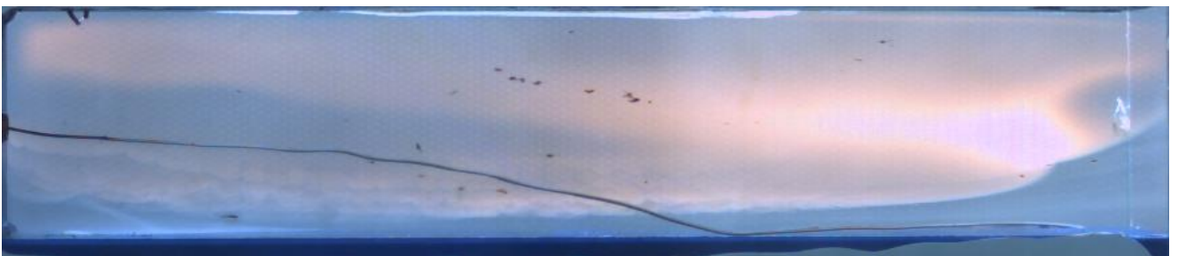
Figure 4-10: Premixed Li-ion LMO-air mixture, with SOC at 30 %. Printscreen of the flame front 0.0475 s from the position in Figure 4-9. The battery is referred to as F37.
