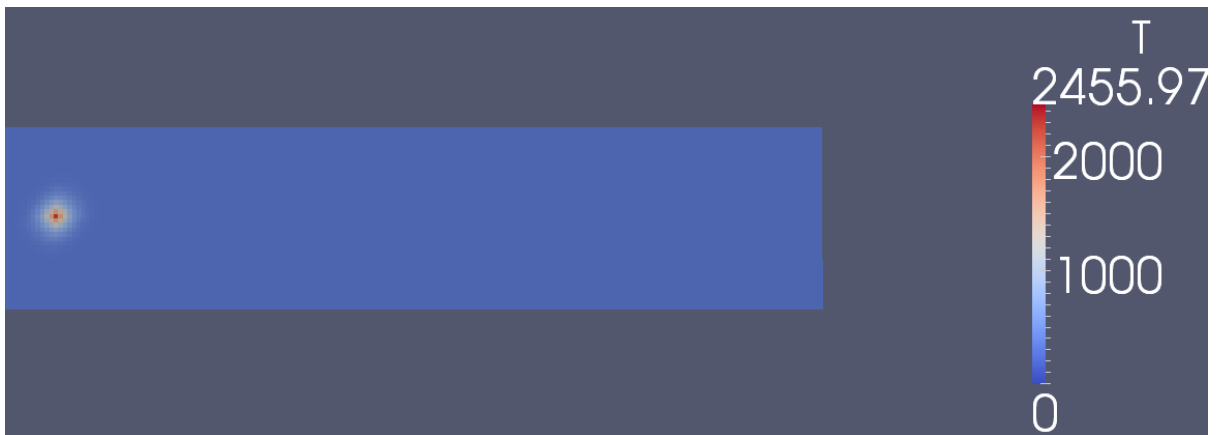
Figure 3-20: Temperature of premixed Li-ion LCO gas-air, at time step: 0.01
