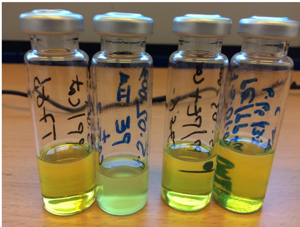
Figure C 1: liquid oil produced from catalytic cracking; from left: PP, LDPE, LDPE/PP (3.4/6.6), and LDPE/PP (6.6/3.4)
