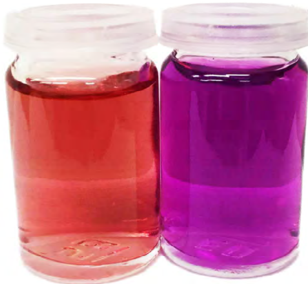
Figur 28 Preliminary BPR and acetic acid experiments. Left glass: BPR, right glass: BPR+Acetate
