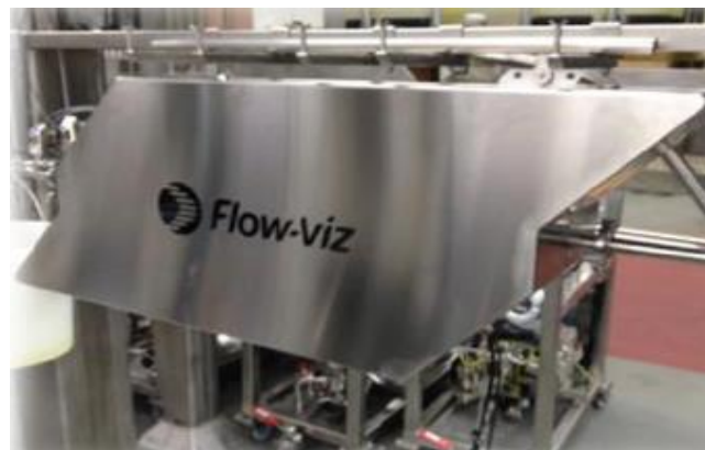
Figure 18: "Flow-viz" - an instrument to measure viscosity for non-Newtonian fluids in real time [17]
