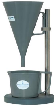
Figure 13: Marsh Funnel instrument
