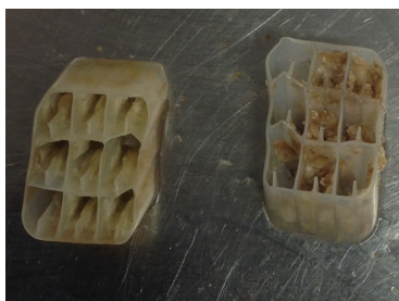
Figure 3–2: Mature BWTS ® biofilm carriers
