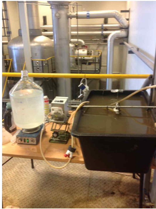
Figure 3: Equalisation tank along with buffer solution pumping setup
