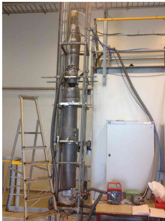
Figure 1: Insulated reactor at NSO along with feed and recycle pump
