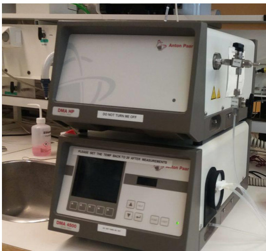
Figure 3A- 3. Anton paar DMA 4500 Density/specific gravity/concentration meter
